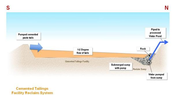
This is a side view of the cemented tailings facility. Cemented paste tails will be pumped into the facility which will have a 1-2 degree flow so that all water will settle out and drain into the gravel and rock. There will be a sump pump here which will be pump the excess water out of the facility to the process water pond.
